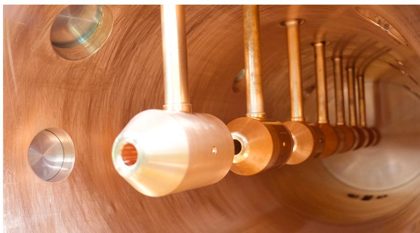
In Sweden, at the ESS, *European Spallation Source*, research centre which will host the world's most powerful neutron source in Lund, the first protons passed through the Drift Tube Linac 1, DTL1, one of the key components of the ESS accelerator built in Italy by INFN researchers.
